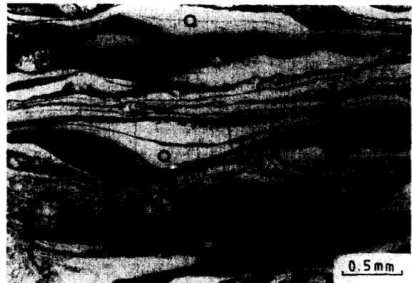
Fig. 2. Microfabric of mylonitized granodiorite with alternating quartz ribbons ( $Q$ ), feldspar aggregates and lensoid biotite clasts ( $b$ ) which define the foliation. A weak shear band cleavage is developed from lower left to upper right.
